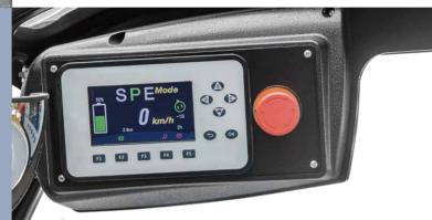
A PIN code should be provided before entering the system. 99 sets of PIN codes are available for the administrator. The truck is highly secured and irrelevant personnel cannot start the truck.
